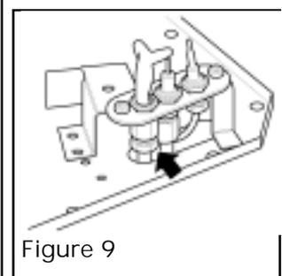
9. Remove the pilot injector. Replace with the LPG injector. See figure 10.
