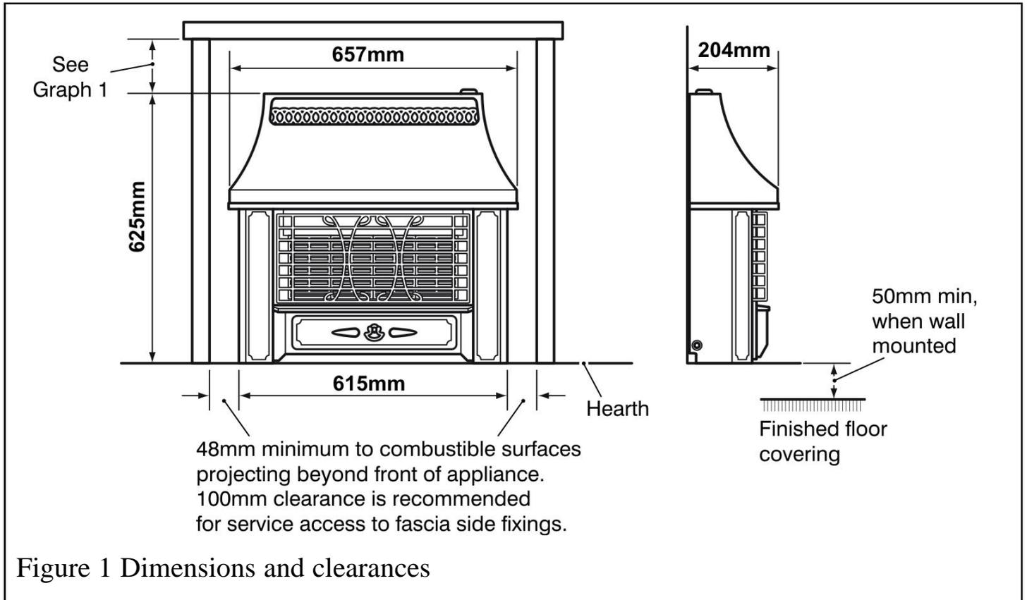
Figure 1 Dimensions and clearances
