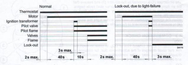
When flame-failure occurs during working, shut down takes place within one second.
