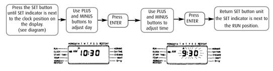
NOTE: When setting the time or altering the temperature settings, if a period exceeding 60 seconds is allowed to elapse between button presses then the CentaurStat will automatically return to the run position. Any alterations made since the last press of the ENTER button will not recognised.
