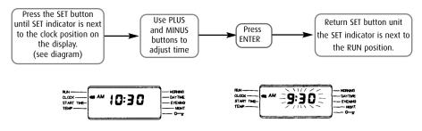
NOTE: When setting the time or altering the temperature settings, if a period exceeding 60 seconds is allowed to elapse between button presses then the CentaurStat will automatically return to the run position. Any alterations made since the last press of the ENTER button will not recognised.
