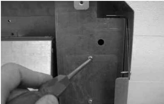
Fig. 12 Control Valve Panel Removal
