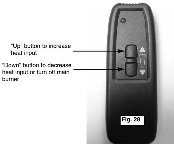
**NOTE :** The remote control does not light the pilot, it only lights the main burner when the pilot flame is established and regulates the heat input between high and low.
