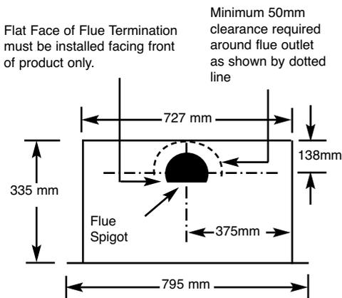
**Side View of Combustion Chamber**
