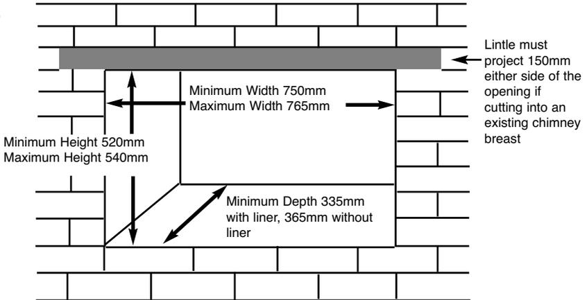
**NOTE :** Please ensure that access holes are cut into either the sides or area above the lintel to allow access to the flue pipe connection if using a flue liner. Such access holes are also advantageous in installations where a flue liner is not required as they provide access for servicing purposes.
