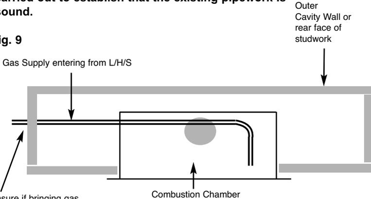
Ensure if bringing gas supply through side or rear of a chimney breast that the pipe is sleeved and sealed with a suitable flexible, non setting compound
