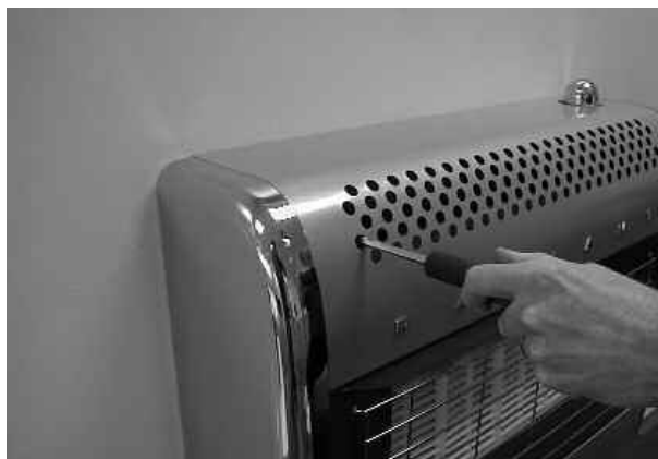
Fig. 4 Remove the Upper Outer Case Fixing Screws
