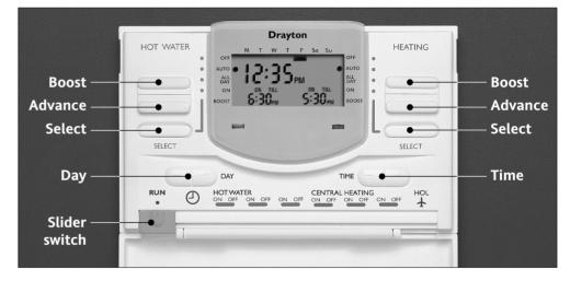
The Tempus 7 electronic programmer will automatically switch ON and OFF up to three times a day. You can select one set of times for weekdays and different times for weekends (5/2 day), or programme different times for each day of the week (7 day). Hot water and heating times can be set independently.
